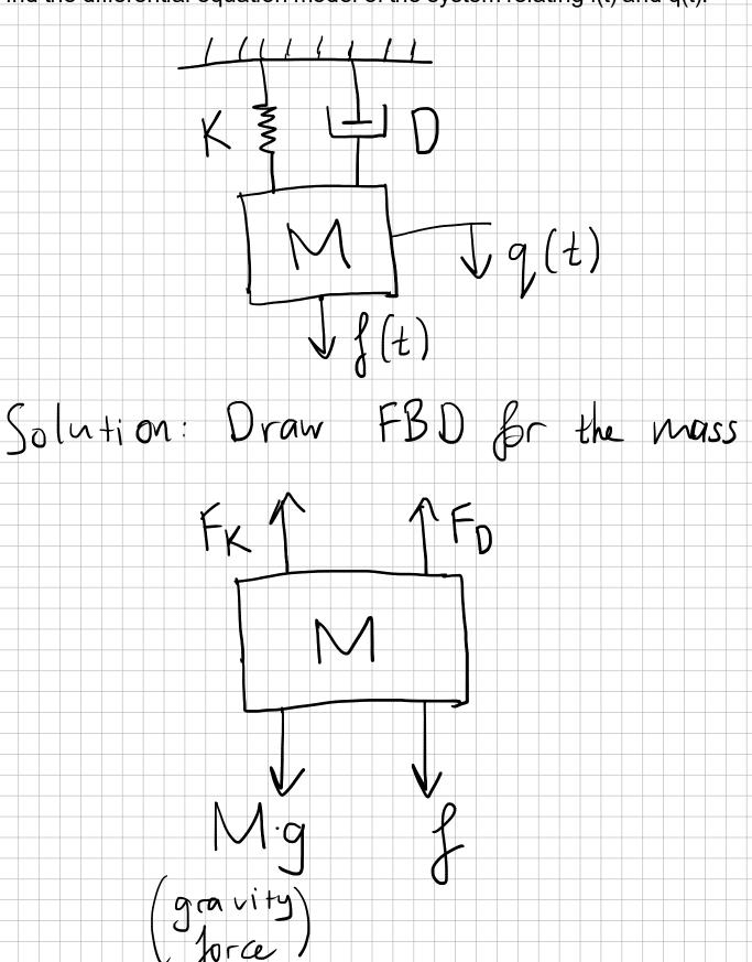
From linear models of spring & damper, we can write: FK = K.9  $F_D = D \cdot \dot{\gamma}$ Writing N2L for the mass:  $\sum_{i} F_{i} = M\alpha = M\ddot{2}$ 8+Mg-K-g-D-g=Mg or (rearranging to have a terms on LHS): [M.j. + D.j. + K2 = f+Mg]
