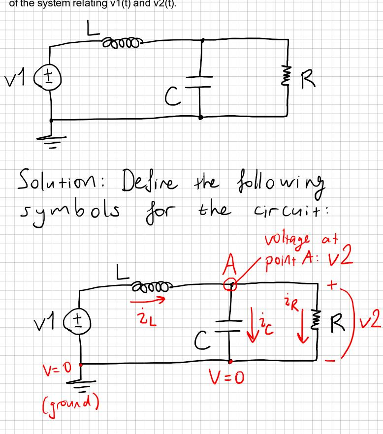
Invoking KCL at point A: il = ic + ir Involving KVL for left Cop:  $\sqrt{1} = \sqrt{L} + \sqrt{2}$ The question asks us to relate V1 and v2, thus we need to rewrite VL and Ve in terms of v2 Writing the linear model of the inductor:  $V_L = L \cdot \dot{z}_L$ Rewriting KVL with this: v1 = L iL + v2
