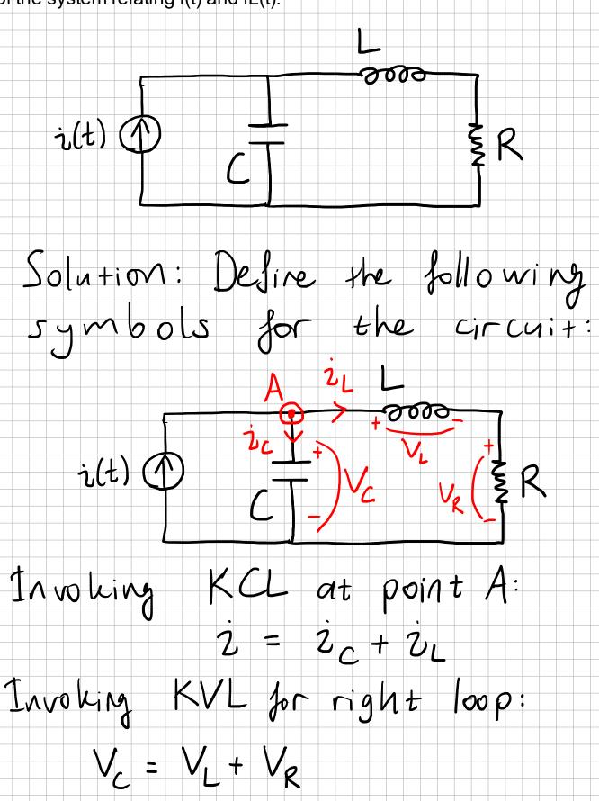
From linear models of the inductor and the resistor, we can write: V<sub>L</sub> = L i<sub>L</sub> V<sub>R</sub> = R i<sub>L</sub> Rewriting KVL with these:  $V_C = L \cdot \dot{z}_L + R \cdot \dot{z}_L$ Differentiating both sides:  $V_c = L \cdot i_L + R \cdot i_L$ Multiplying both sides by C: TC. Vc = L.C. iL + R.C. i From linear model of the capacitor: ic = C. Vc IThis equation thus be comes: Lic = L·C·iL+R·C·iL
