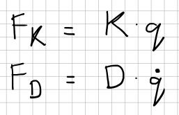
Writing N2L for the mass:  $\sum_{i} F_{i} = M\alpha = M\ddot{g}$  $f - K \cdot q - D \cdot \dot{q} = M \ddot{q}$ or (rearranging to have g terms on LHS):  $\left| M \cdot \ddot{q} + D \cdot \dot{q} + K q = \beta \right|$
