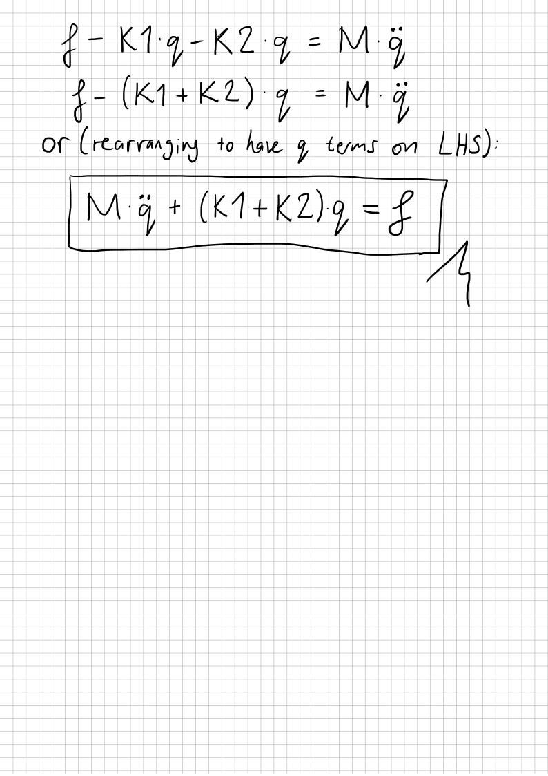
Question 3: Consider the schematic of a translational mechanical system depicted below, consisting of a mass, a spring, and a damper (with parameters M, K, and D, respectively). Position of the mass is denoted as q(t). An external force is being applied to the system, denoted as f(t). Gravity is acting on the system, with gravitational acceleration constant g. There are no other forces acting on the system. Find the differential equation model of the system relating f(t) and q(t).
